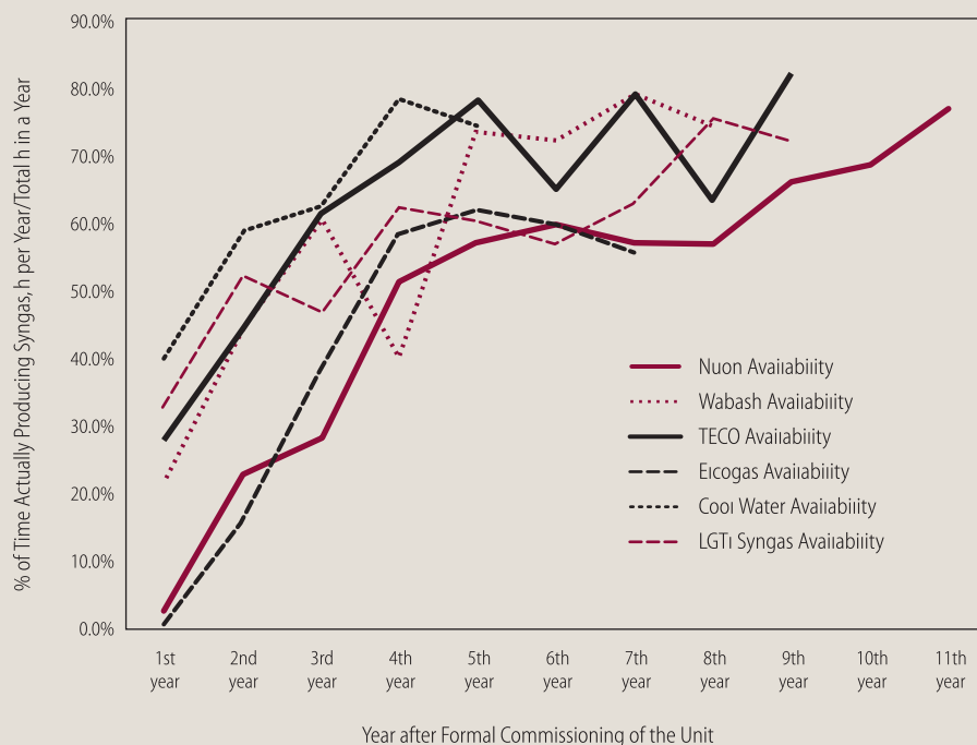
Figure A-3.B.13 History of IGCC Availability for the Start-up of Coal-based Units (excluding operation on back-up fuel)
